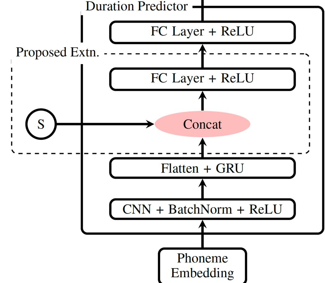
Block diagram of the duration predictor with the proposed extension, 'S' stands for speaker embedding.
