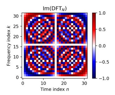
The matrix DFT<sub>N</sub> and a visualization of its real and imaginary parts for the case N = 32
