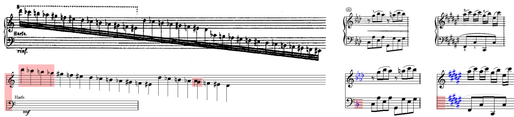
■ Figure 6 Examples of common OMR errors. Left: Besides wrong note durations and an accidental mistaken for a note, the staff system was split into two systems. Middle: The key signature was not correctly recognized for the lower staff. Right: In the lower staff, the clef was not detected.
