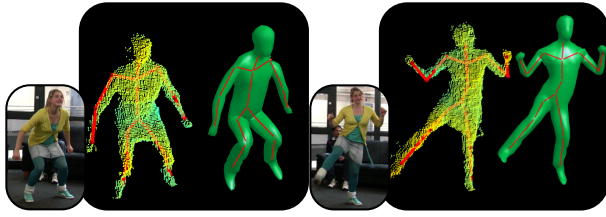
Figure 7. In case of slightly different body proportions, we can simply scale M_i to roughly match our body model.
