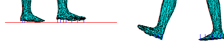
Figure 7. Integration of the constraint foot on floor . Points on the sole are pushed onto the floor.
