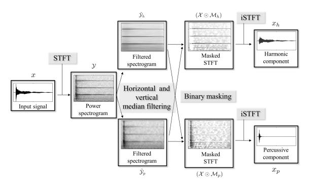
Figure 3: Harmonic-percussive source separation.
