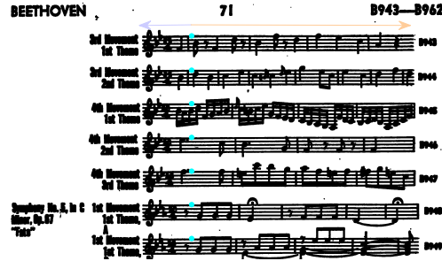
Figure 2.9: L and R positions are located by searching a white pixel in the directions marked from any one of the detected y-coordinate (blue).
