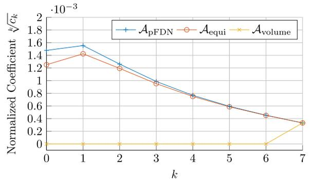
Fig. 5. Normalized coefficient of the absolute echo density and its approximations with  $\mathbf{m} = [479, 587, 673, 773, 881, 991, 1091, 1201]$  and  $N = 8$ .
