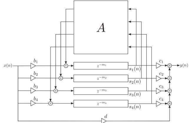
Fig. 1. Feedback delay network structure for artificial reverberation as proposed by Stautner and Puckette [12].
