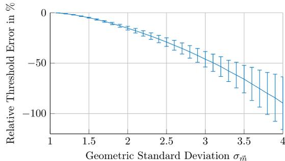
Fig. 4. Mean relative threshold error (solid) and error standard deviation (error bars) of  $(t_{\text{equi}} - t_{\text{pFDN}}) / t_{\text{pFDN}}$  between the equilateral approximation  $\mathcal{A}_{\text{equi}}$  and the absolute echo density  $\mathcal{A}_{\text{pFDN}}$  for  $N = 8$ .
