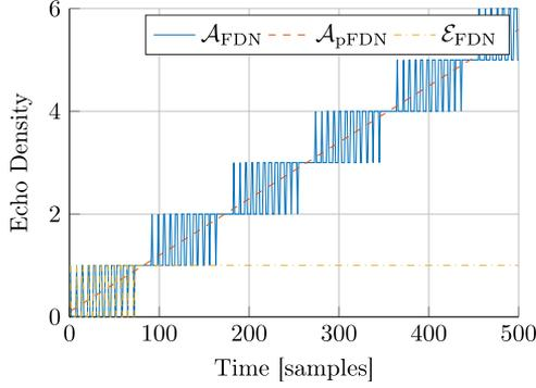
Fig. 3. Absolute, polynomial absolute, and empirical echo density for FDN with  $N = 2$  and delays  $\mathbf{m} = [7, 13]$ . Absolute and empirical echo densities are identical up to the point of saturation  $t_{\text{sat}} = 73$ . The polynomial part  $\mathcal{A}_{\text{pFDN}}(n)$  is given by (21).
