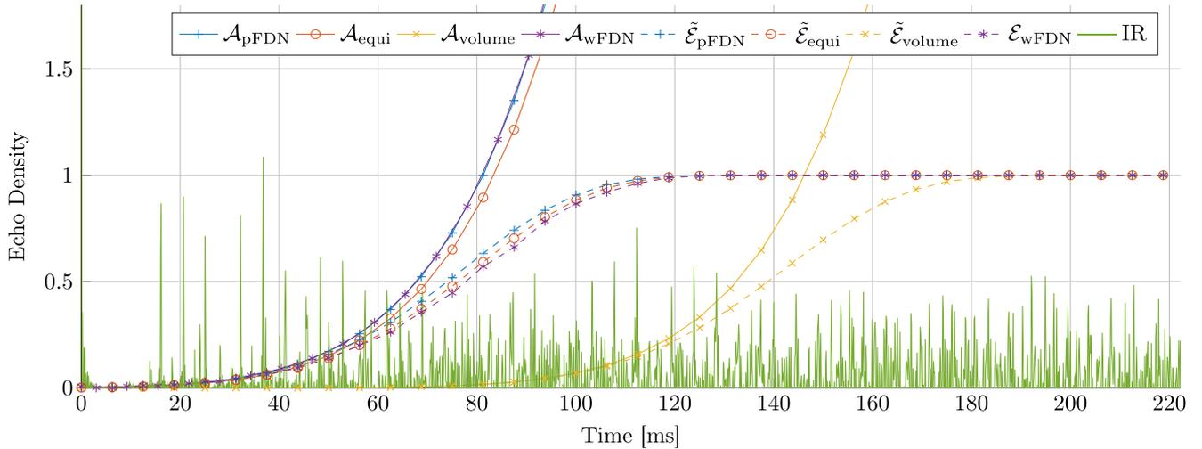
Fig. 7. Absolute echo density and the volume and equilateral approximations (solid lines) with  $\mathbf{m} = [479, 587, 673, 773, 881, 991, 1091, 1201]$  and  $N = 8$ . The expected empirical echo densities are added along side the smoothed empirical echo density (dashed lines). The absolute value of the impulse response is added for reference.
