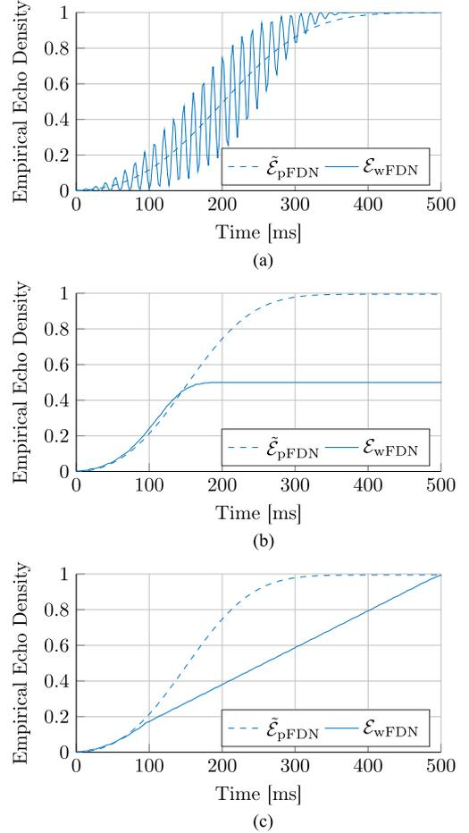
Fig. 6. Examples of degenerated delays  $\mathbf{m}$ . (a) Clustering:  $m = [635; 657; 627; 1321]$ . (b) Common Primes:  $m = [308; 558; 908; 1022]$ . (c) Low-order Dependency:  $m = [307; 557; 907; 1021]$ .
