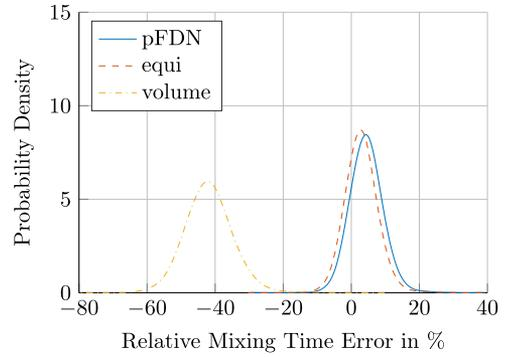
Fig. 9. Probability density function of the relative mixing time error  $\epsilon_{\text{Abel}}$  based on a Monte Carlo simulation.
