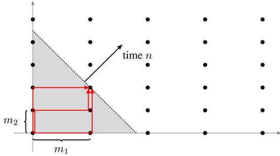
Fig. 2. Echo lattice of an FDN with  $N = 2$  and  $\mathbf{m} = [m_1, m_2]$ . The dots indicate the coordinates of the echoes in terms of the delay lengths. The red arrows indicate three paths  $\mathbf{p} = [2, 2, 1]$ ,  $[2, 1, 2]$  and  $[1, 2, 2]$  with the same echo time  $n_{\mathbf{p}}$ . The dotted line indicates the expanding time polygon, whereas the gray shaded triangle indicates the time simplex.
