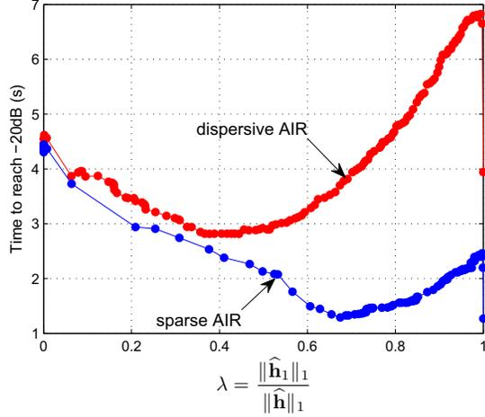
**Fig. 2.** Time to reach -20 dB normalized misalignment level for different values of  $\lambda$  in (14) for PB-IPNLMS using the input signal generated by (16). Impulse response in Fig. 1 (b) and (c) were used as sparse AIR and dispersive AIR respectively. [ $\mu = 0.3$ , SNR = 20 dB]
