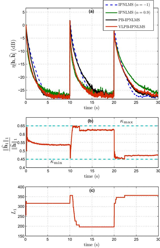
**Fig. 3.** **a)** Relative convergence of IPNLMS for  $\alpha = -1$  and 0.9, PB-IPNLMS with proportionate weight allocation technique [4] and VLPB-IPNLMS; **b)** evolution of  $\frac{\|\hat{\mathbf{h}}_1(n)\|_1}{\|\hat{\mathbf{h}}(n)\|_1}$ ; **c)** evolution of  $L_1$ ; The input signal was generated using (16) with an echo path change at 10 s and 20 s, from that shown in Fig. 1 (a) to (b) and then to (c),  $\mu = 0.3$  and  $\text{SNR} = 20$  dB.
