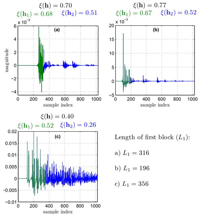
**Fig. 1.** Acoustic impulse responses obtained using the method of images [7].  $\xi(\mathbf{h})$ ,  $\xi(\mathbf{h}_1)$  and  $\xi(\mathbf{h}_2)$  respectively denote the sparseness measures [8] of the full impulse response, the first block with size  $L_1$  and the second block.
