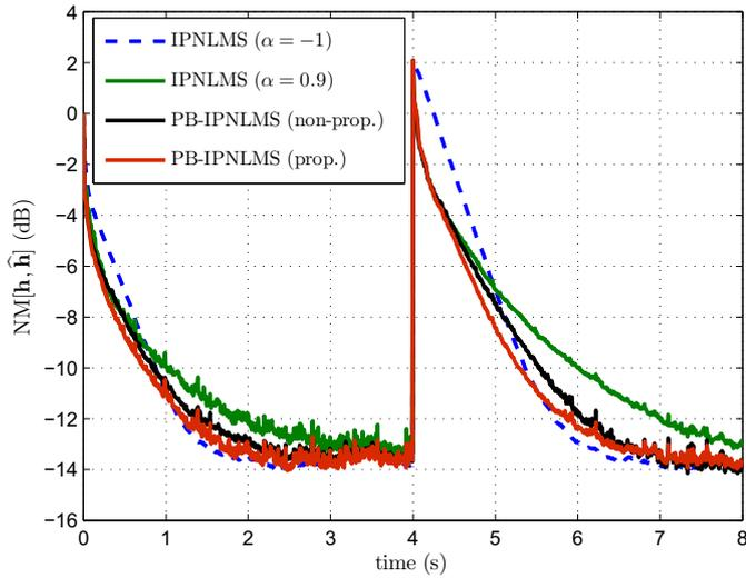
Fig. 5. Relative convergence of IPNLMS for  $\alpha = -1$  and 0.9 and PB-IPNLMS with non-proportionate and proportionate weight allocation approaches, using WGN input signal with an echo path change at 4 s. Impulse response is changed from that shown in Fig. 1 (a) to (b) and  $\mu = 0.3$ , SNR = 20 dB.
