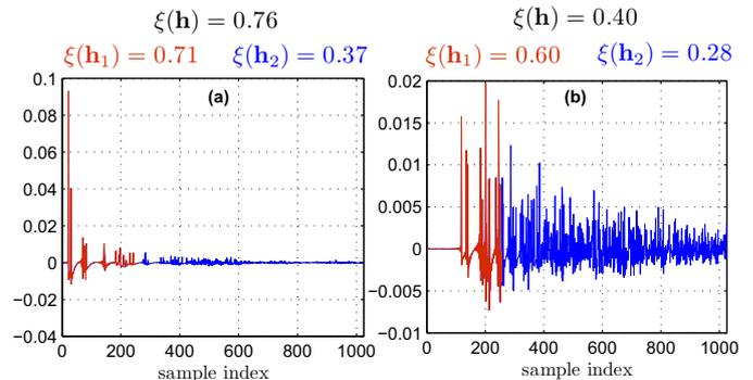
Fig. 1. Acoustic impulse responses obtained using the method of images [9].  $\xi(\mathbf{h})$ ,  $\xi(\mathbf{h}_1)$  and  $\xi(\mathbf{h}_2)$  respectively denote the sparseness measures [6], [10] of the full impulse response, the first block with size of 256 and the second block.
