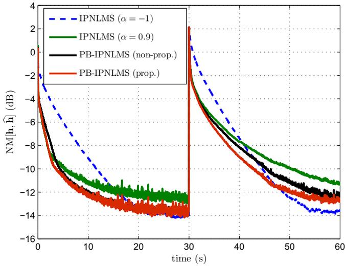
Fig. 8. Relative convergence of IPNLMS for  $\alpha = -1$  and 0.9 and PB-IPNLMS with non-proportionate and proportionate weight allocation approaches, using the input signal generated by (18) with an echo path change at 4 s. Impulse response is changed from that shown in Fig. 1 (a) to (b) and  $\mu = 0.3$ , SNR = 20 dB.
