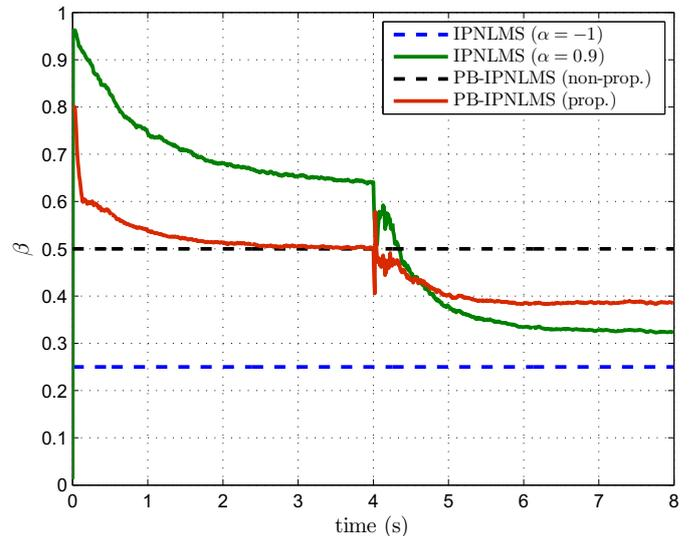
Fig. 7. Evolution of  $\beta$  in (16), which is equivalent to  $\|\hat{\mathbf{h}}_1(n)\|_1$  for the IPNLMS algorithm with  $\alpha = -1$  and  $\alpha = 0.9$  and 0.5 for the non-proportionate PB-IPNLMS algorithm.
