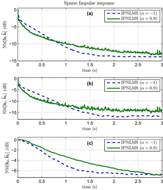
Fig. 3. Normalized misalignments (NM) of IPNLMS with different mixing parameters,  $\alpha$ , for identification of a sparse impulse response.
