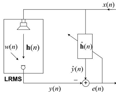
Fig. 2. Adaptive system for acoustic echo cancellation in a Loudspeaker-Room-Microphone system.
