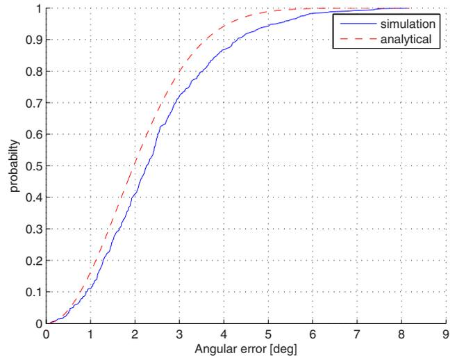
FIG. 6. (Color online) Comparison of theoretical and simulated (image-source method) AE cumulative distribution functions.
