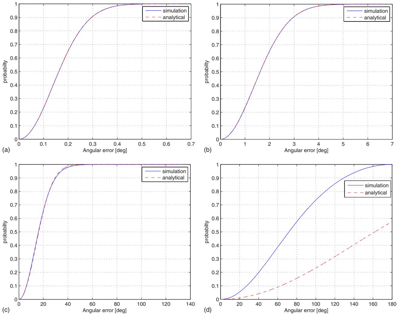
FIG. 5. (Color online) Sample cumulative distribution function of angular error (produced with extended Polack model) compared to function predicted by analytical analysis of  $\tilde{\delta}_{\text{asym}}$  for various levels of  $\text{DRR}_{E_s}$ .
