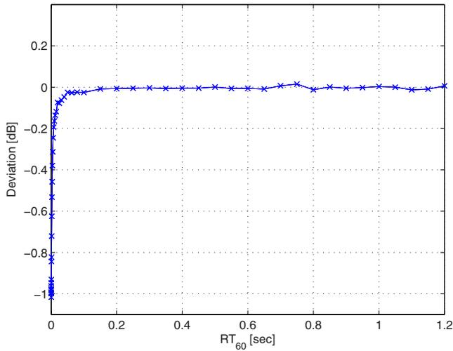
FIG. 3. (Color online) Deviation of theoretical value of  $E\{\mathbf{IAV}[0]\}$  from the sample mean obtained by Monte Carlo simulation results, as a function of the  $RT_{60}$ .
