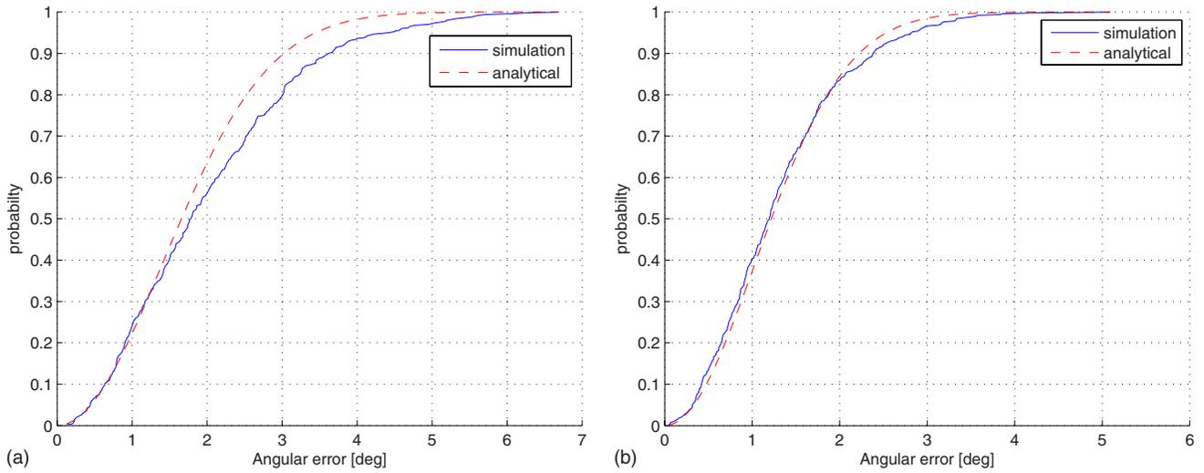
FIG. 7. (Color online) Comparison of theoretical and simulated AE cumulative distribution functions when early arrivals are removed.
