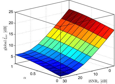
**Fig. 4.** The normalized global noise-reduction factor obtained using a coherent plus non-coherent noise field  $i\text{SNR}_c = \{-5, \dots, 30\}$  dB ( $i\text{SNR}_{nc} = 20$  dB,  $T_{60} = 0.3$  s,  $N = 4$ ,  $D = 2$  m).
