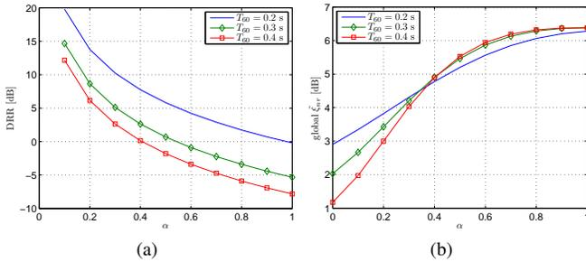
**Fig. 3.** a) The DRR of  $Q(j\omega, \alpha)$  for  $T_{60} = \{0.2, 0.3, 0.4\}$  s. b) The normalized global noise-reduction factor obtained using  $T_{60} = \{0.2, 0.3, 0.4\}$  s ( $N = 4$ ,  $D = 4$  m,  $i\text{SNR}_{nc} = 5$  dB).
