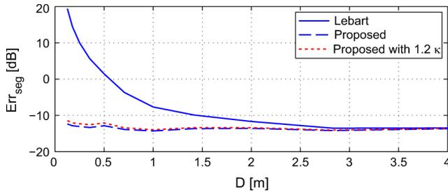
Fig. 2. Mean segmental error ( $\text{Err}_{\text{seg}}$ ) calculated using all speech signals from the APLAWD database for Lebart's (solid), the proposed estimator with  $\hat{\kappa} = \kappa$  (dashed) and  $\hat{\kappa} = 1.2\kappa$  (dotted) as a function of the source-microphone distance  $D$ .
