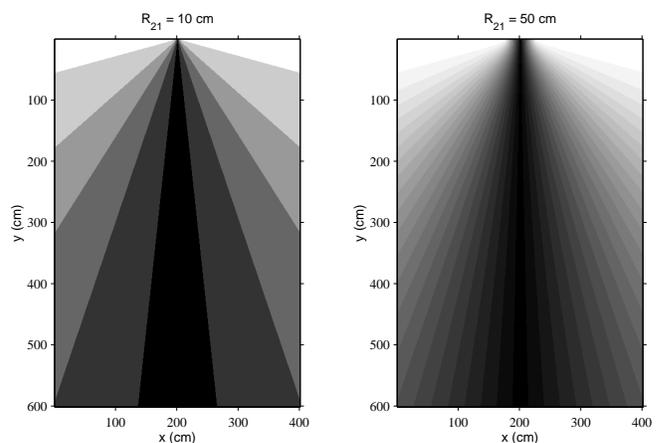
Fig. 3. Range differences at 16 kHz for different inner microphone distances.
