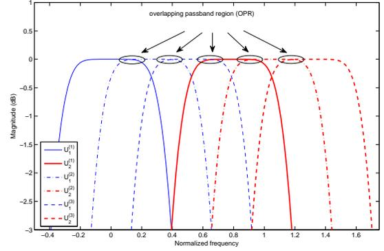
Fig. 1. Multiple filterbanks showing the OPRs.
